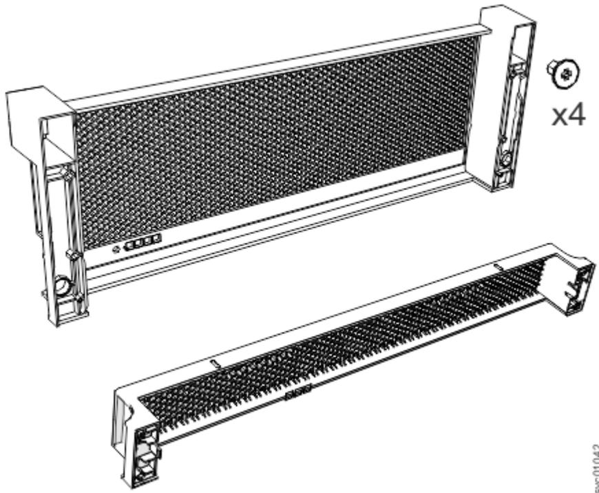
Figure 95. Fascia components on the expansion enclosure
