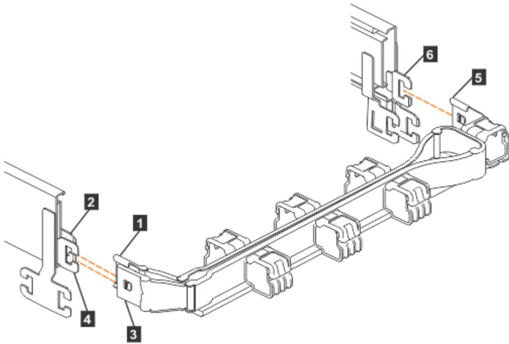
Figure 73. Connectors for the cable management arm
