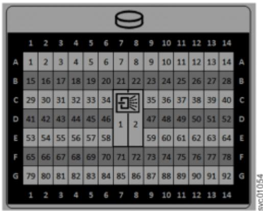
Figure 111. Drive locations in a 2145-92F expansion enclosure
