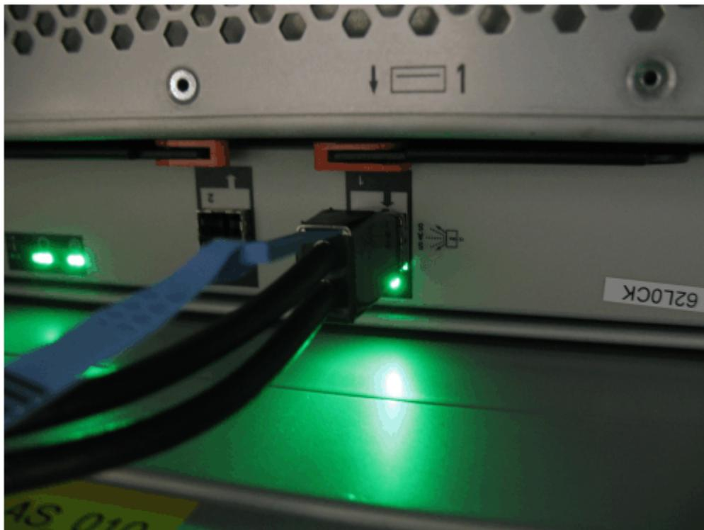
Figure 100. SAS cable correctly inserted into the SAS port
