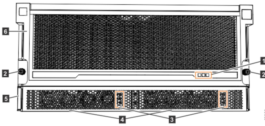
Figure 44. Features on the front of the 2145-92F expansion enclosure
