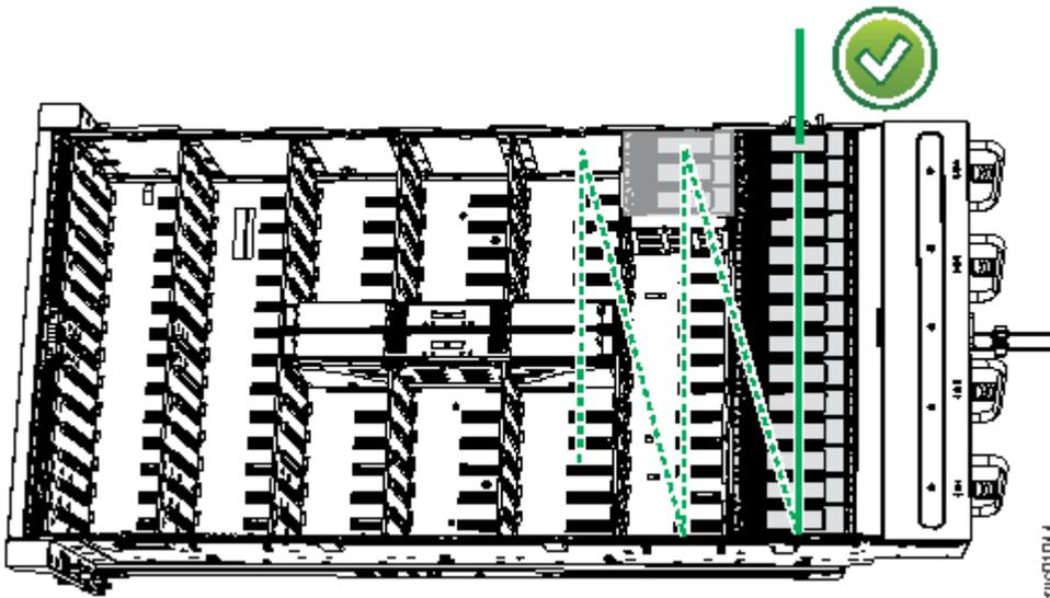
*Figure 83. Correct drive installation*
