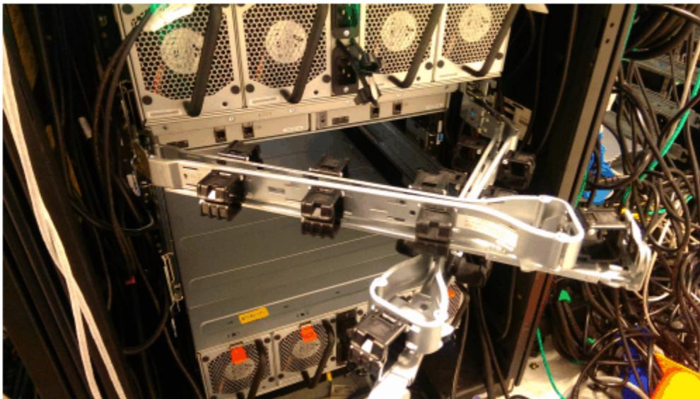
Figure 67. Upper and lower CMA assemblies moved aside
