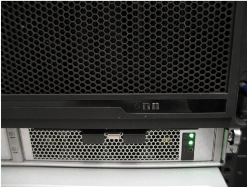
Figure 97. Fascia removed from the PSUs
