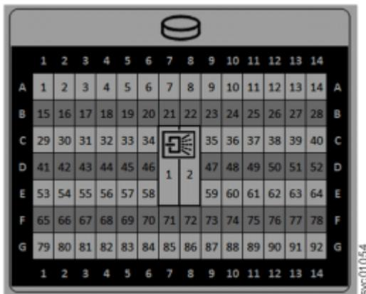
Figure 82. Drive locations in a 5U expansion enclosure
