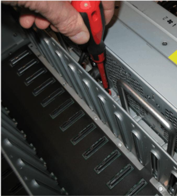
*Figure 125. Loosen the FIB screws*
