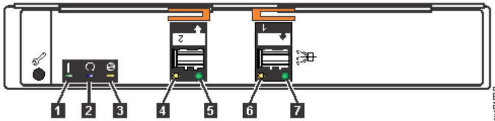
Figure 118. Expansion canister
