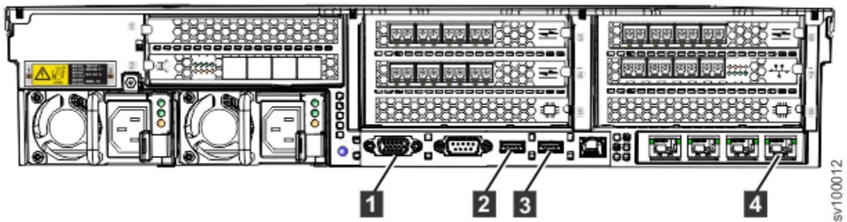
Figure 15. SAN Volume Controller 2145-SV1 service ports
