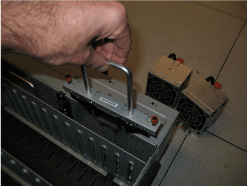
*Figure 104. Insert the new FIB in the chassis*
