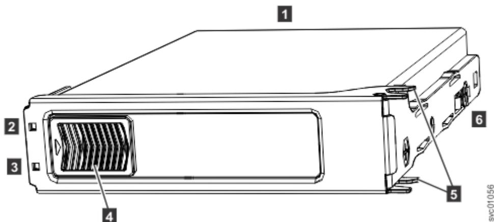
Figure 144. LEDs on a drive assembly
