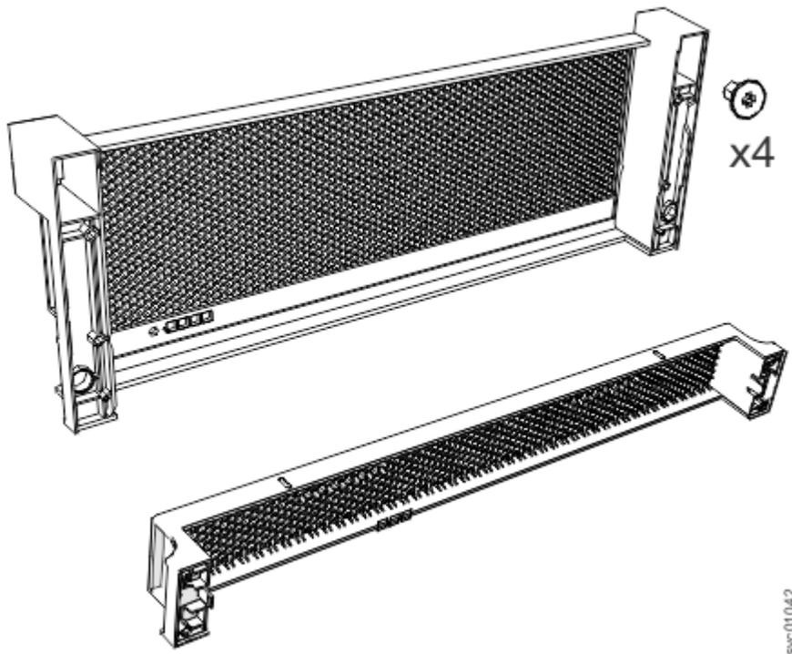
Figure 90. Fascia components on the expansion enclosure
