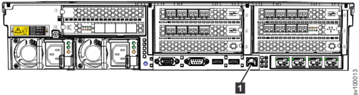
Figure 16. SAN Volume Controller 2145-SV1 unused Ethernet port
