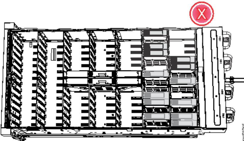
*Figure 84. Incorrect drive installation*
