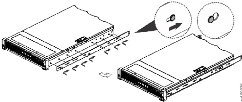
Figure 23. Attach inner rail section to chassis
