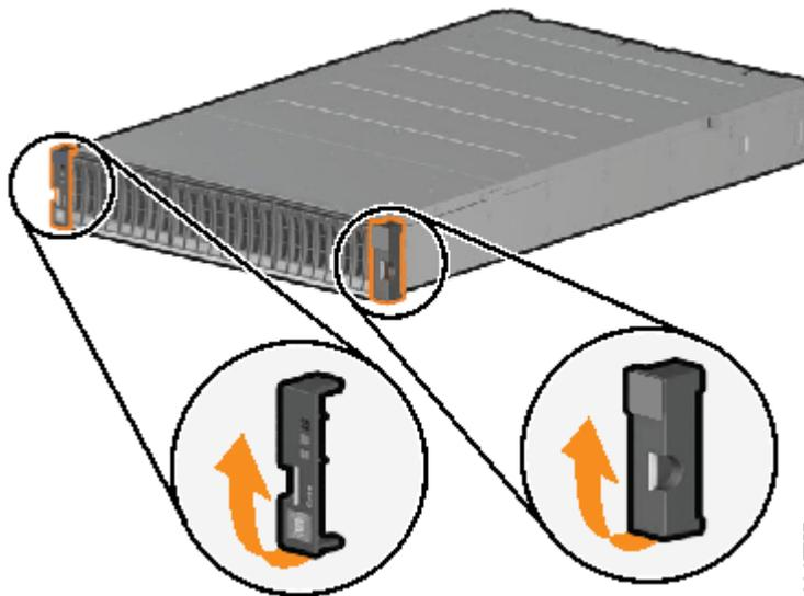
*Figure 40. Removing enclosure end caps*
