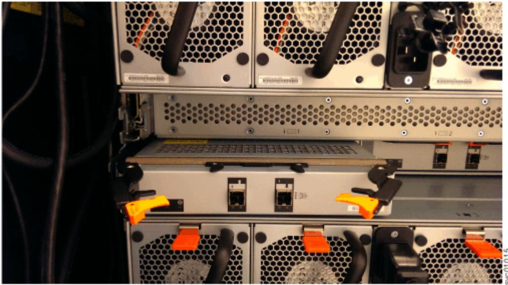
Figure 119. Removing the expansion canister
