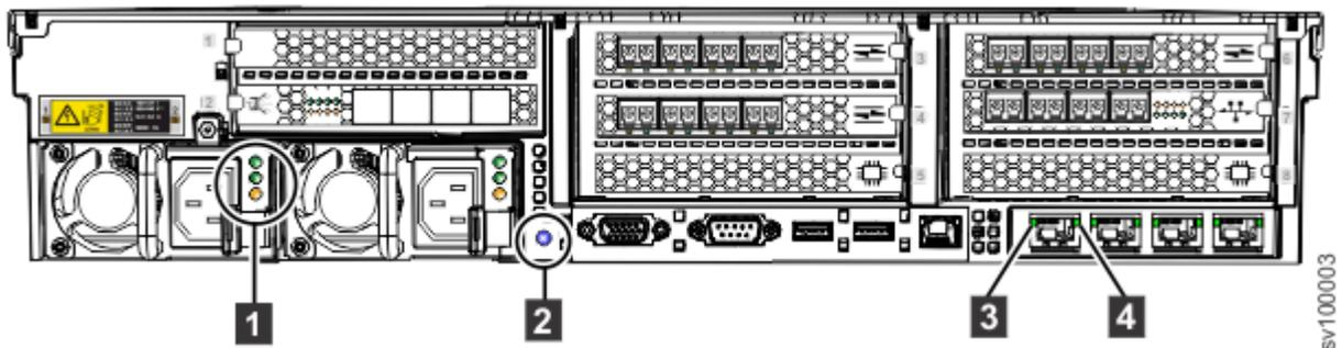
Figure 3. SAN Volume Controller 2145-SV1 rear-panel indicators
