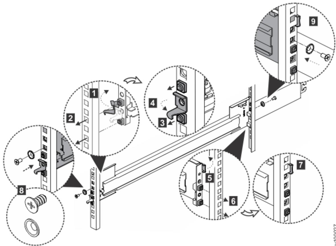
Figure 24. Install the bracket assembly to the frame
