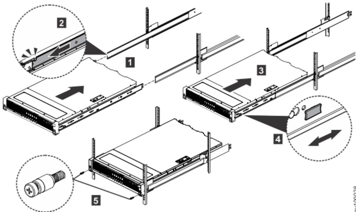
Figure 25. Insert the chassis into the rack
