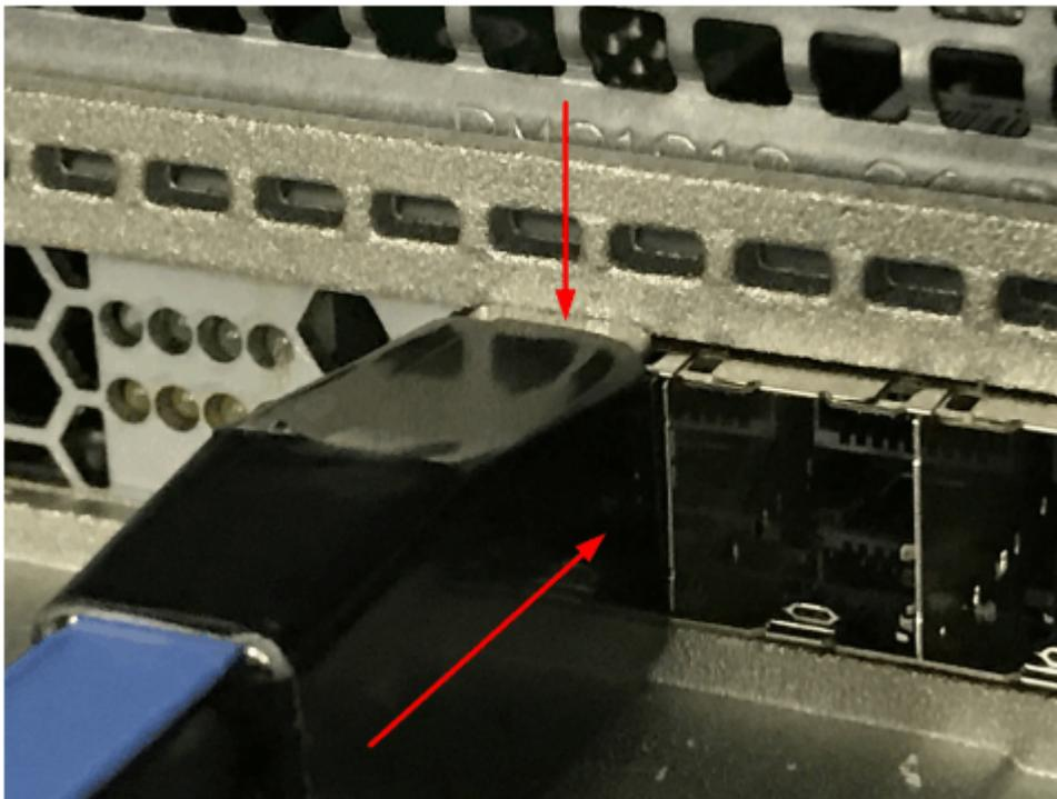
Figure 135. Pushing the SAS cable latch closed
