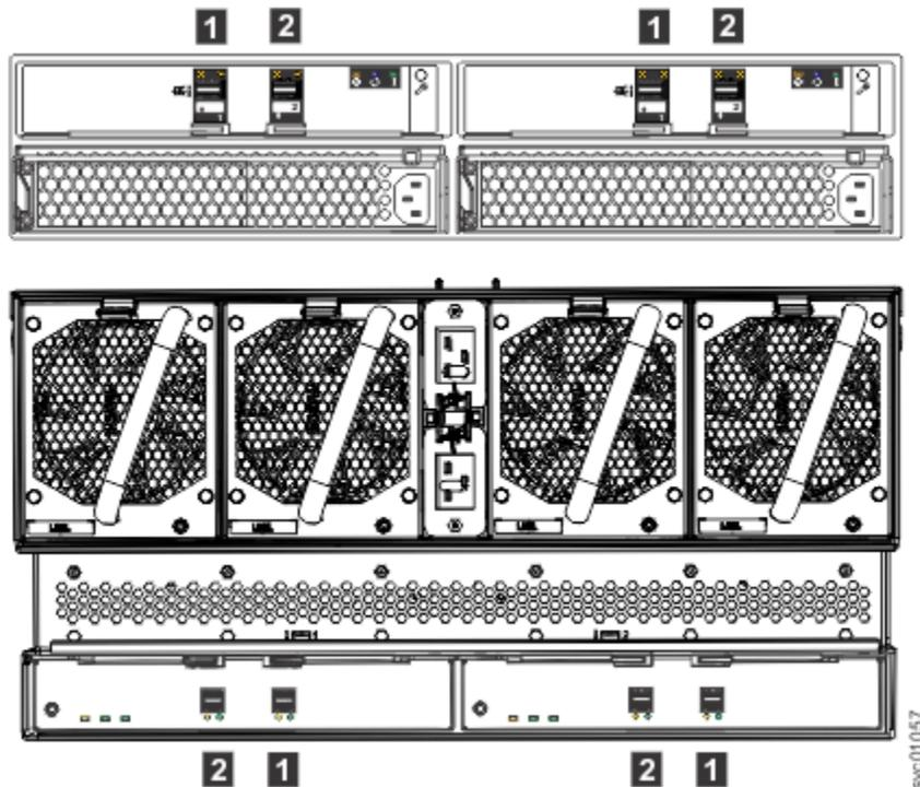
Figure 137. SAS port orientation on expansion enclosures
