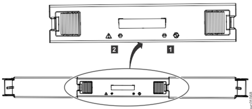
Figure 145. LEDs on a secondary expansion module
