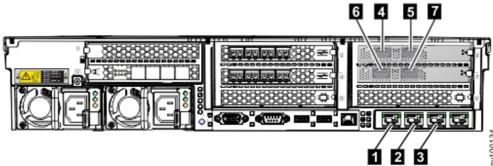
Figure 19. Ethernet port numbers for 25 Gbps adapter
