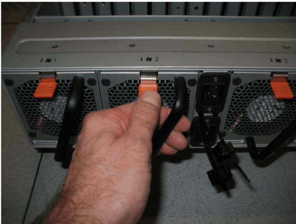
Figure 121. Fan module release tab
